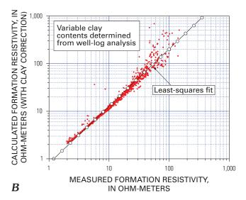
**Figure 6.** Plots showing clay-corrected resistivity versus observed resistivity at the Mallik 2L-38 well, Mackenzie Delta, Canada. Archie constants for shaly sand are  $a^* = 1.02$  and  $m^* = 1.95$ , and for a clean sand they are a = 1 and m = 2. The resistivity of connate water was set to 0.25  $\Omega$ ·m. A, Using constant clay contents (average of 30 percent). B, Using variable clay contents from well-log analysis.
