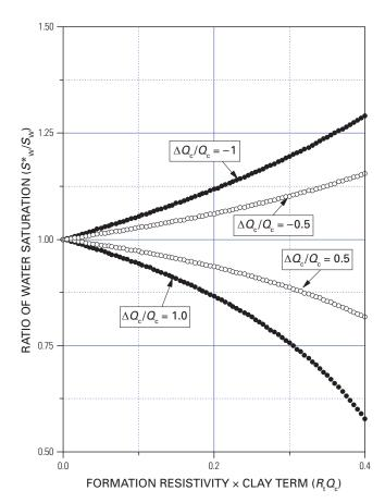
**Figure 8.** Graph showing the ratio of water saturation versus the formation resistivity times the clay term  $(R_{tac})$  for different relative errors in the clay term  $(Q_c)$ .  $S_w$  is the water saturation estimated from the resistivity when there is no error in  $Q_c$ , and  $Q_c$  is the estimated water saturation when there is a relative error in  $Q_c$ . Solid dots indicate an error of 100 percent, and open circles are errors of 50 percent.
