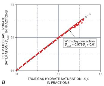
**Figure 5.** Plots showing estimated gas hydrate saturation ( $S_{h,est}$ ) versus true gas hydrate saturation ( $S_h$ ) for the model shown in figure 4A. A, Without clay correction. B, With clay correction.
