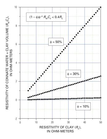
**Figure 3.** Graph showing relationship between the resistivity of clay  $(R_c)$  and the product of connate-water resistivity  $(R_w)$  and clay volume  $(\mathcal{C}_v)$  required to yield an approximate linear relationship between log resistivity and log porosity. The values under each curve satisfy the linearity condition.
