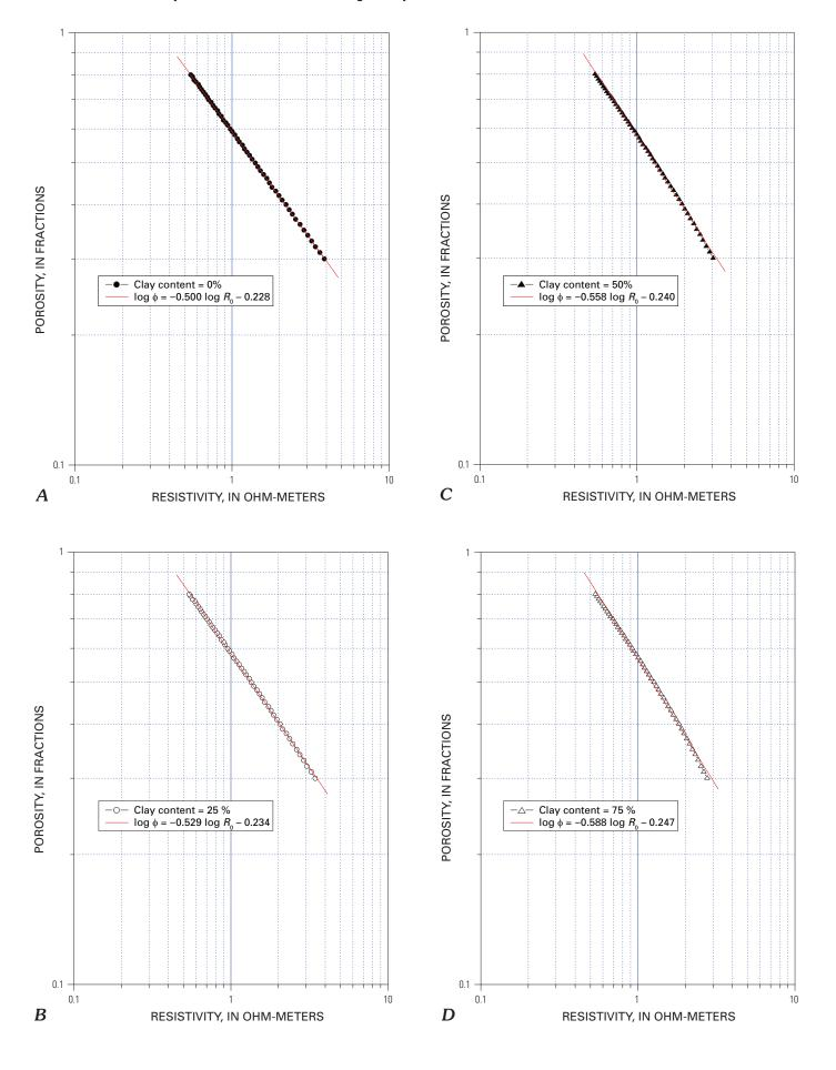
**Figure 2 (previous page).** Plots of logarithm of the porosity versus logarithm of the resistivity to show the linear relationship. The model parameters are identical to those for figure 1A, which are a=1, m=2, water resistivity ( $R_{\rm w}$ ) = 0. 35  $\Omega \cdot$ m, and clay resistivity ( $R_{\rm c}$ ) = 5  $\Omega \cdot$ m. Plots are for A, clean sand; B, 25 percent clay; C, 50 percent clay; and D, 75 percent clay.
